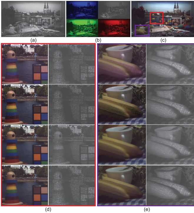
Fig. 11. Indoor scene with structured NIR illumination. The denotation of (a)-(e) is the same as in Fig. 8, except that in each close-up, the columns correspond to color channels, first column for RGB and second column for NIR. Four rows correspond to: bilinear upsampling (first row), Martinello et al. (second row), Tang et al. (third row) and the proposed method (fourth row).
