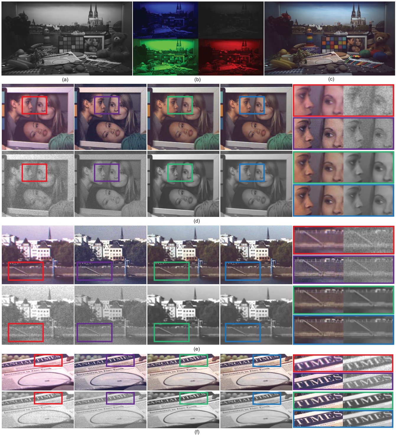
Fig. 10. Indoor scene without structured NIR illumination. (a) Captured raw image of an indoor scene, (b) extracted color channels, (c) the reconstructed RGB image of the proposed method. We compare reconstructions of bilinear upsampling, Martinello et al. (second column), Tang et al. (third column), and the proposed method (fourth column) of RGB (first row) and NIR (second row) channel respectively. The smaller close-up are shown on the right of each figure for further comparison.
