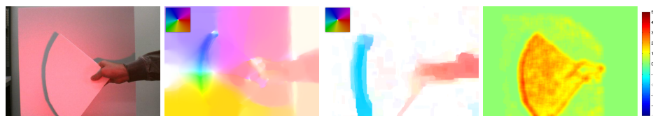
Figure 7.15: Failure case of optical flow for a moving, but untextured scene (left). Optical flow [252] and SIFT flow [253] for two succeeding color frames are shown in the second and third column; the 2D flow vectors are color-coded with the shown color wheel (insets). Both methods cannot recover the true 2D motion of the fan and wrongly segment the scene. Our orthogonal velocity estimate can resolve this problem and properly segment the scene.
