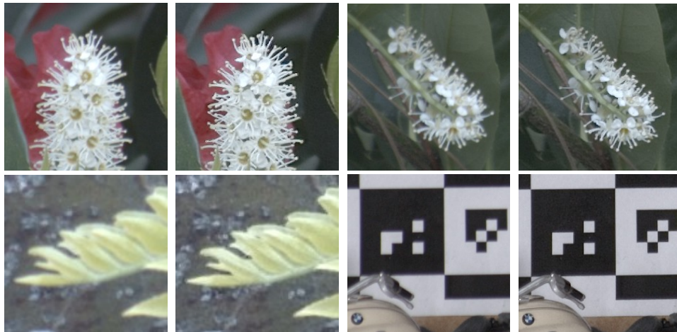
Figure A.18: Patches from an image captured with a commercial Canon lens (105 mm, f/4.5 ). First and third column: Captured input patches. Second and last column: reconstructed sharp result.
