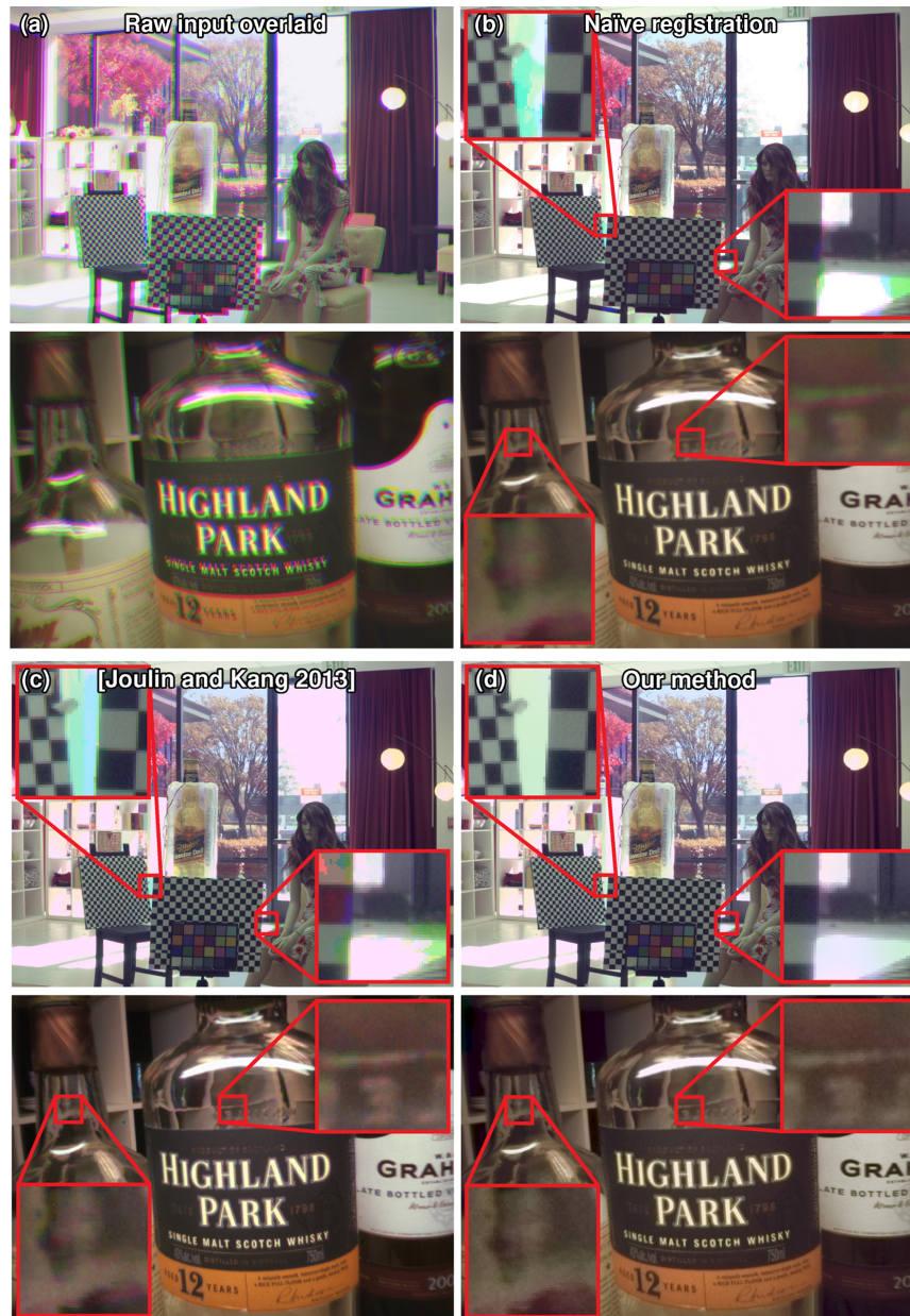
Figure A.27: Image reconstruction for color-array camera. (a) Raw input red, green, and blue images overlaid. (b) Naïve registration of color channels via optical-flow produces color leaks. (c) Anaglyph-based reconstruction [328] partially reduces the color leakage. (d) Our method reconstructs the image without such artifacts.
