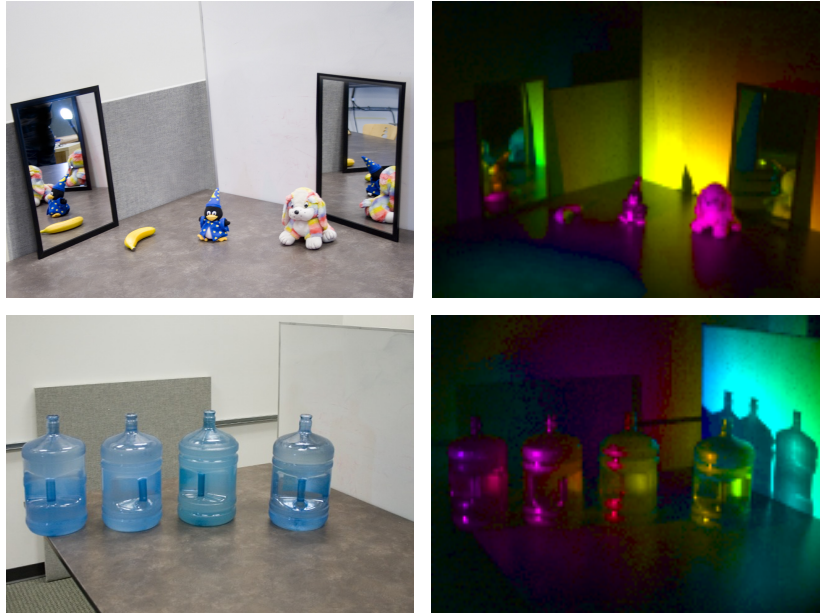
Figure 3.8: Our test scenes, in addition to the one from Figure 3.1. All scenes are illuminated from the left, with the rainbow images encoding the temporal location of the main intensity peak for each pixel. Top: Various objects on a table, and their reflections in mirrors placed nearby. Note how the items and mirrored counterparts light up at different times. Bottom: Four bottles filled with slightly scattering water. The specular reflections reach the camera before the light scattered inside the bottles.
