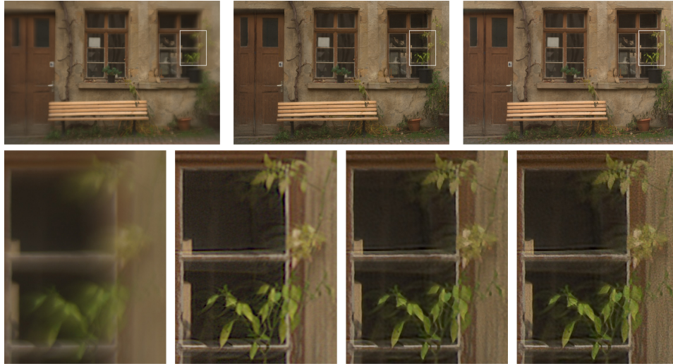
Figure A.21: Top row from left to right: Captured image, our deconvolved result, result from [165]. Patch matrix below from top left to bottom right: Captured image, result from [165], our result with strong regularization (smoother reconstruction), our result with low regularization (more detailed reconstruction).
