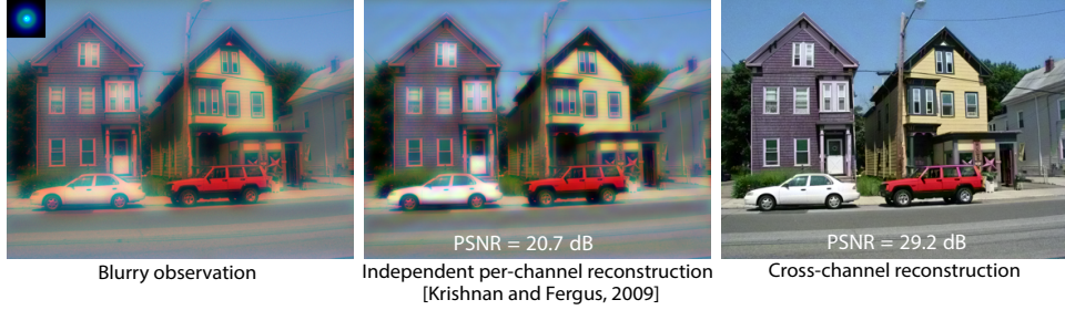
Figure 8.3: Effect of using the cross-channel prior for a simulation using a strongly chromatic blur (in the very top left) Left: Blurred and noisy observation. Middle: Independently deconvolved results for each channel using [160]. Right: Deconvolution with our cross channel prior.
