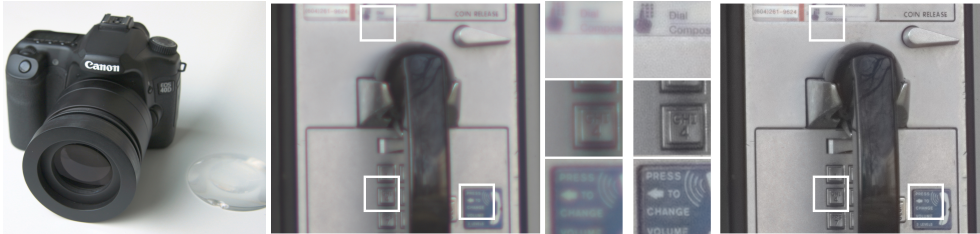
Figure 8.1: High-quality imagery through poorly performing lenses: Relying on the specific structure of chromatic aberrations, we present a Bayesian reconstruction method for the removal of aberrations post-capture. This enables imaging using simple lenses that suffer from severe aberrations. From left to right: Camera with our lens system containing only a single glass element (the plano-convex lens lying next to the camera), unprocessed input image, result estimated using the proposed approach.
