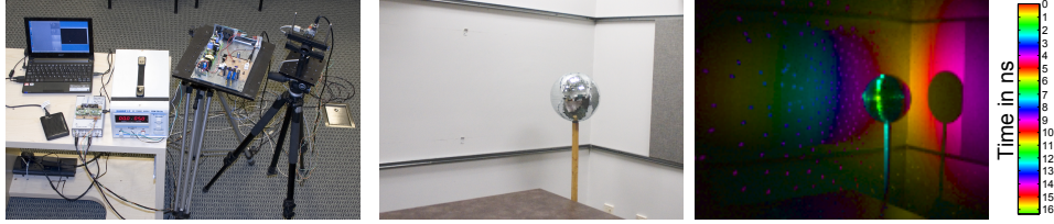
Figure 3.1: Left: Our capture setup for transient images (from left: computer, signal generator, power supply, modulated light source, CIS camera). Middle: A disco ball with many mirrored facets. Right: The same sphere as seen by our transient imager when illuminated from the left, colored according to the time offset of the main intensity peak.
