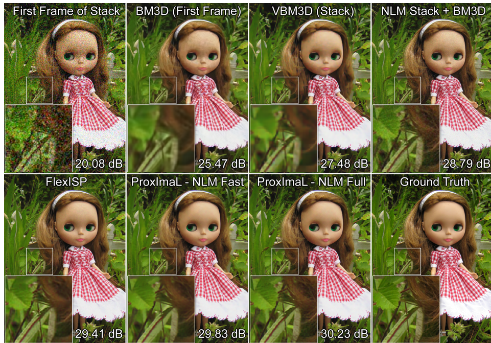
Figure 10.8: Comparison of image priors for burst denoising & demosaicking. For this simulation, a non-local means (NLM) prior outperforms the BM3D prior. The approximate NLM implemented in OpenCV is faster than, but not quite as good as, a full implementation.
