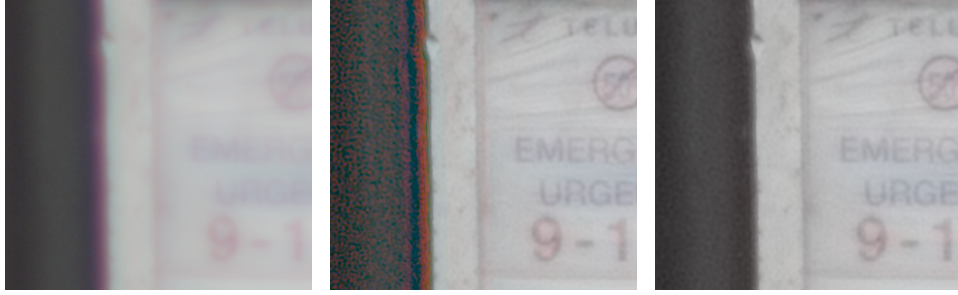
Figure 8.5: Chromatic artifacts in low-light areas. Left: Original blurred patch captured with a plano-convex lens. Center: Reconstruction using Eq. (8.4). Notice the chromatic artifacts in all low-intensity areas and the correct reconstruction in the other areas. Right: Regularization for low-intensity areas added as discussed below.
