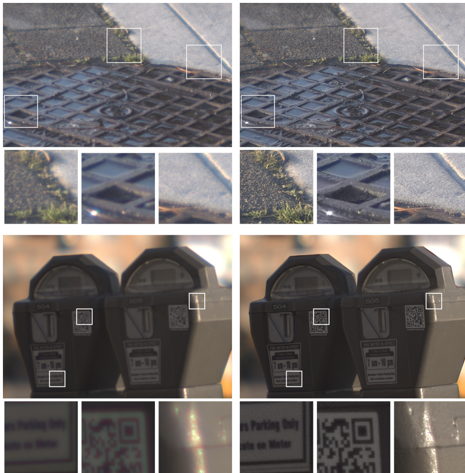
Figure 8.6: Images captured with a simple plano-convex lens (left) and restored with our method (right). Note recovered spatial detail and the absence of color fringing. Also note the bokeh and graceful handling of out-of-focus blur in the top three images.
