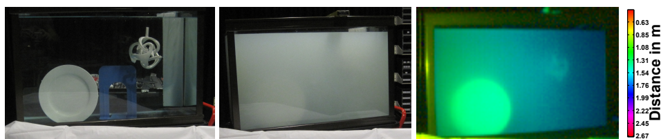
Figure 4.1: Example of imaging in scattering media using our approach. Left: Original scene with objects submerged in water-filled glass tank. Center: 160 ml milk added. Right: Objects that are “invisible” due to strong scattering, like the structured object on the top right or parts of the circular object become detectable using our approach.
