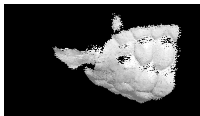
(d) After a few seconds of scanning, the front part of the turtle has been covered relatively well. However, the user sees a few remaining holes.
