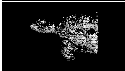
Figure 1: Our real-time 3D model acquisition system was used to scan a small turtle figurine. The total scanning time was 4 minutes and the final model, at 0.5 mm. resolution, contains approximately 200,000 polygons. (c) through (e) are rendered using splats, and (f) is rendered as a polygon mesh.
