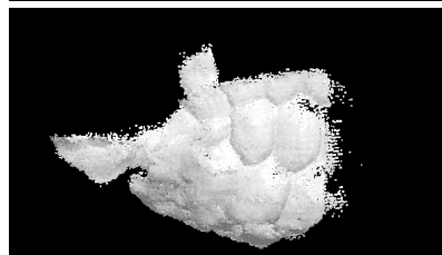
(e) The user turns the object to fill the holes. The user may try a number of different positions until the holes are filled – immediate feedback is available about the effectiveness of each orientation.
