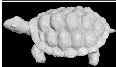
Figure 1: Our real-time 3D model acquisition system was used to scan a small turtle figurine. The total scanning time was 4 minutes and the final model, at 0.5 mm. resolution, contains approximately 200,000 polygons. (c) through (e) are rendered using splats, and (f) is rendered as a polygon mesh.
